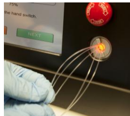
Automatic calibration of all the delivery fibers at one time.
